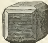
Bevelment of the edges of a cube by planes of a tetrahedron.
